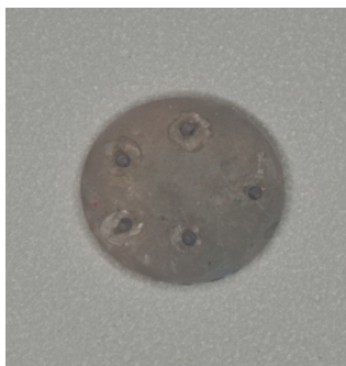
Fig 2. Preparation of specimen for micro-shear bond test
